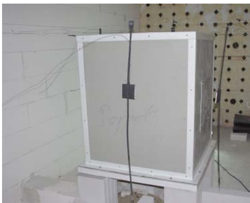
Valve Fire Shelter before start of test
