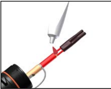
3a. Apply a liberal amount of RTV sealant to cable.
