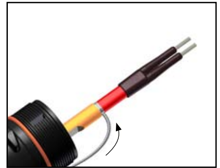
3c. Slide ground sleeve over twisted braid.
